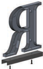
3B - Bottom & Top Rail Mount Letters 4-24, Minimum 3/8 thick Includes painted or anodized c-channel rails. Letters over 8 may require tie-back (not supplied).
