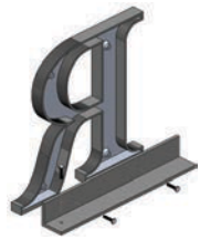
3D - Bottom Back Angle Bracket Mount Letters 4-24, Minimum 3/8 thick. Letters over 12 may require tie-back (not supplied). Angle iron is 2 x 2 with a painted finish.
